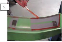
Place the supplied (4) foam squares over the threaded insert holes as shown. Then remove the backing from the double sided tape.
