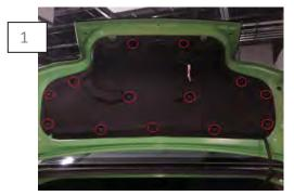
Using a panel removal tool, remove the various push pins and rubber bumpers holding on the trunk lid panel.
