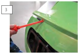
Close the trunk. The spoiler is held down with double sided tape. Using a plastic chisel, gently pry the spoiler free of the trunk lid. \*\*Note: the sheet metal is soft and you can easily scratch/dent the deck trunk. Once the spoiler is removed, clean any excess adhesive off the trunk.
