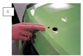
Once the deck lid is clean and free of adhesive, wipe down the surface with the supplied alcohol wipe followed by the adhesion promoter.
