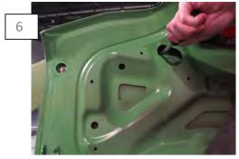
With help, line up spoiler mounting holes with the decklid holes. Using the supplied screws and washers, tighten down the spoiler. Then apply firm pressure on all the tape ledges.
